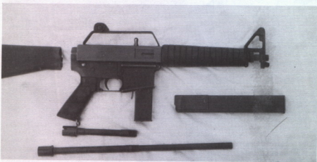
A 9mm conversion unit on an AR-15/M16 lower receiver shown with a detachable butt stock; 16-, 10- (mounted), and 6-inch barrels; and 15- and 30-round magazines. Using an original M16 receiver to make a 6-inch-barrel pistol is making a "short-barreled rifle" according to the BATF.
