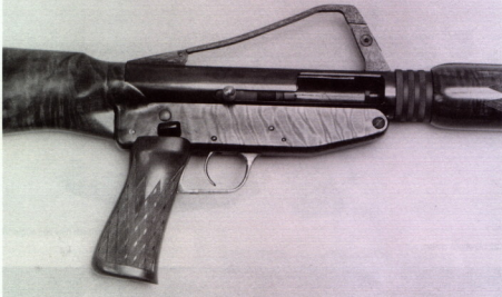
Self-opening trap gun action.
