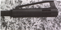
Steel-tube muzzle brake with adjustable front sight.
